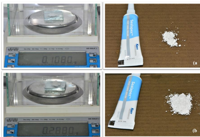
Figure (1): Using analytical balance for weighing (a) 3% of CHNPs. (b) 8% of CHNPs.
