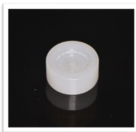
Figure (2): Teflon mold for setting time measurement, fabricated according to ISO standardization 6876:2012.
