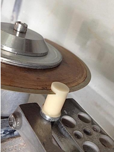
Figure (1): Cutting ceramic discs using Isomet 4000 Linear precision saw machine.
