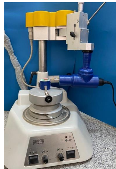
Figure (2): Parallellometer used for polishing procedure holding the mold containing ceramic sample and T-shape attachment with low-speed handpiece fixed inside it.
