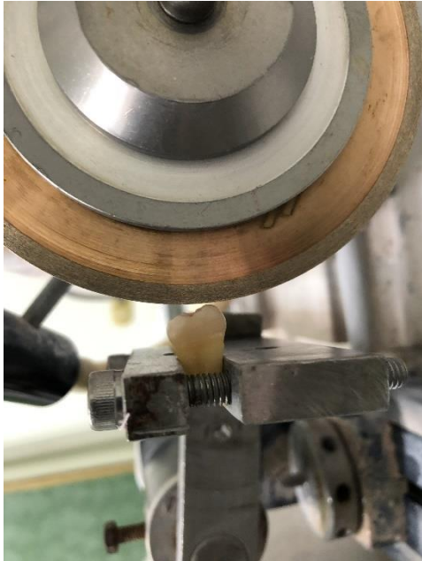
Figure 1: Mounting of samples on Isomet 4000 Clamp.
