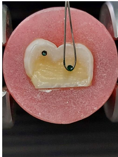
Figure 9: Wire Component around composite microcylinder for \mu SBS testing.
