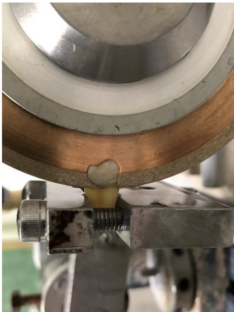
Figure 2: Peeling of buccal enamel of mounted samples.
