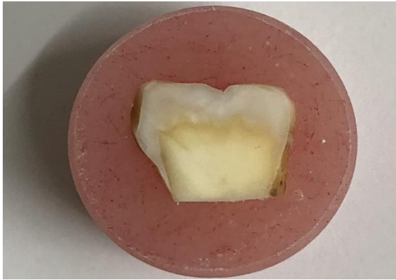
Figure 5: Cold cure acrylic resin containing specimen with enamel peeled off after removal of sectioned PVC pipes.
