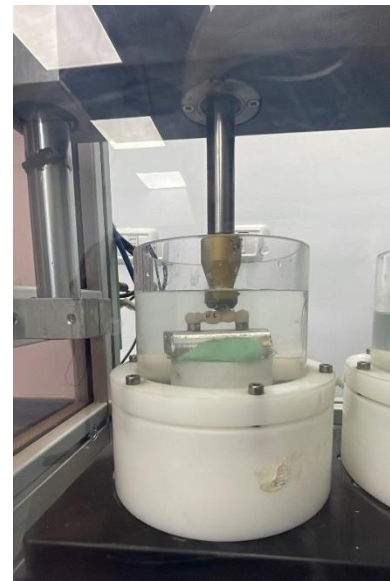
Figure (3): Specimen under cyclic loading.
