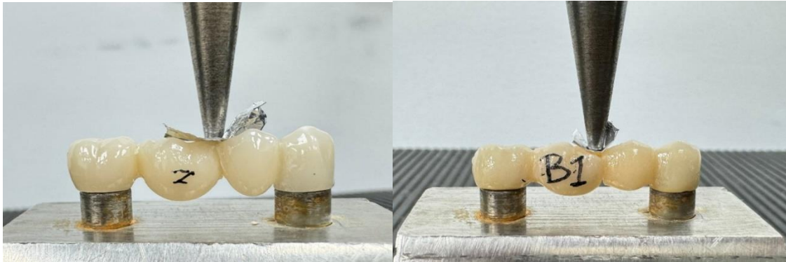
Figure (4): Gradient zirconia 5Y-TZP and 3Y-TZP, and bilayered zirconia 3Y-TZP fracture resistance testing.
