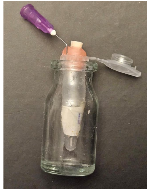
Figure (2): Photograph showing the debris collection apparatus.
