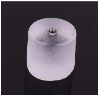
Figure (1): The implant fixture in the middle of the epoxy resin block.
